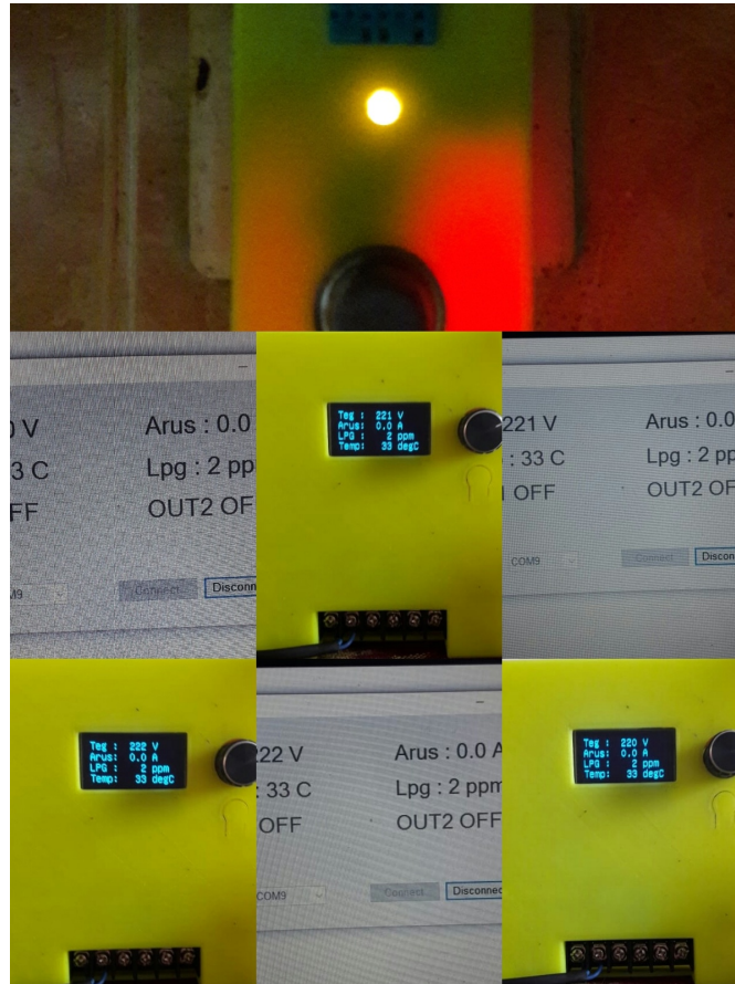
FIGURE 9. A prototype of LPG gas leak detection system
